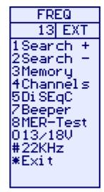
Search +/-) A signal search can be initiated by using the keypad '1 Search +' to search with increasing frequency or '2 Search -' with decreasing frequency. The search mode moves to the next peak in the spectrum and attempts a lock for DVB-S QPSK, DVB-S2 QPSK and DVB-S2 8PSK signals. The symbol rate is determined automatically. Because the time to lock for low symbol rate signals increases the lower the symbol rate, symbol rate signals below about 16000 will not lock during a search.
