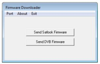
Select the RS232 port on the computer. Normally, the port is COM1 but sometimes the USB to RS232 adapter will use some other port. If desirable, this USB to RS232 adapter can be made to always use COM1 by clicking Control Panel / Device Manager / Ports and in the Advanced settings for the adapter set to COM1.
