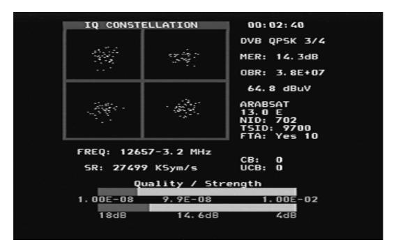
This shows a typical constellation from a DVB-S QPSK signal. The frequency and offset are shown below the constellation diagram and the measured symbol rate is shown below the frequency. The two thermometer bars show the BER and SNR of the signal. The SNR thermometer increases from right to left and the BER thermometer gets smaller from right to left, so that the best signal is shown by a longer white bar.
