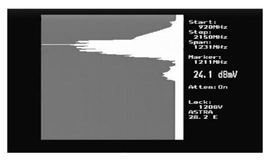
Remember that the displayed UniCable band is reflected in frequency about the User Band frequency as shown in the example below. For more details see Appendix D.
