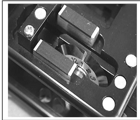
**Figure 33. Fixed blade in position 1 (see the digit on the cleaver)**
