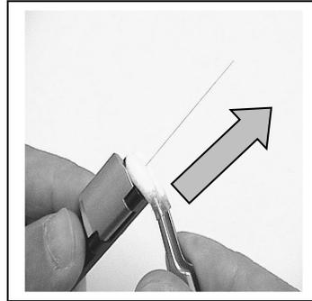
**Figure 15. Cleaning the stripped fiber**
