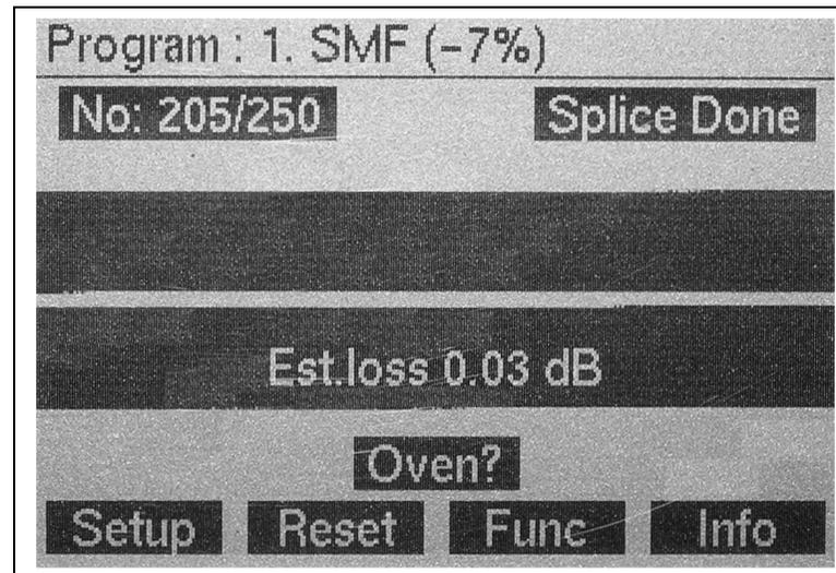
**Figure 24. A finished splice**
