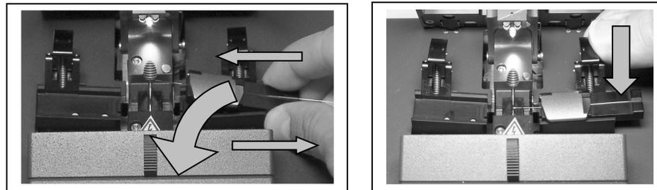
**Figure 18. Insertion of the fiber holder in the fusion splicer**
