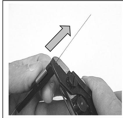
**Figure 14. Stripping the fiber**
