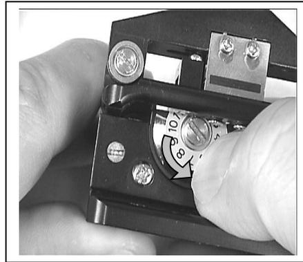
**Figure 30. Rotation of the cleaver blade**
