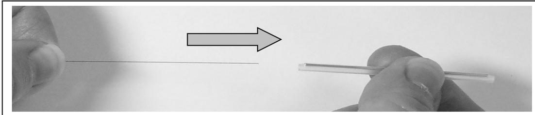
**Figure 13. Introduction of the protecting sleeve**
