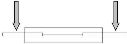
**Figure 26. (a) Schematic picture of a protective sleeve moved into proper position covering the splice.**
