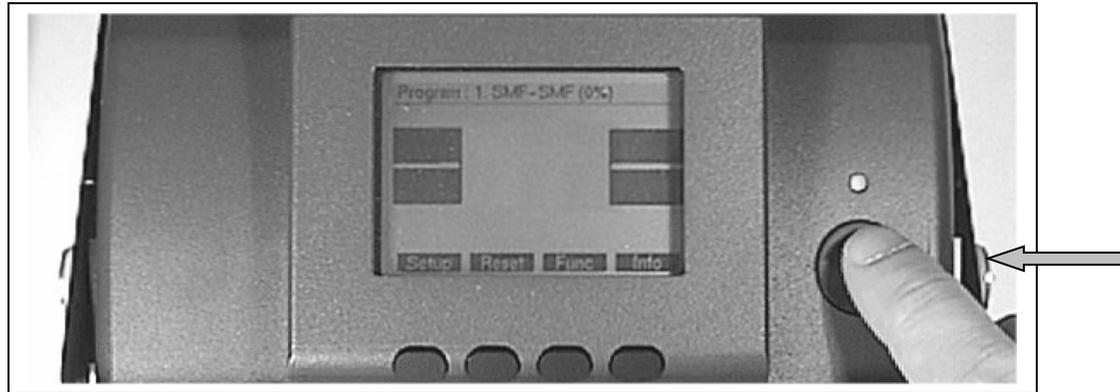
**Figure 23. Splice button for initialization of the splicing process**
