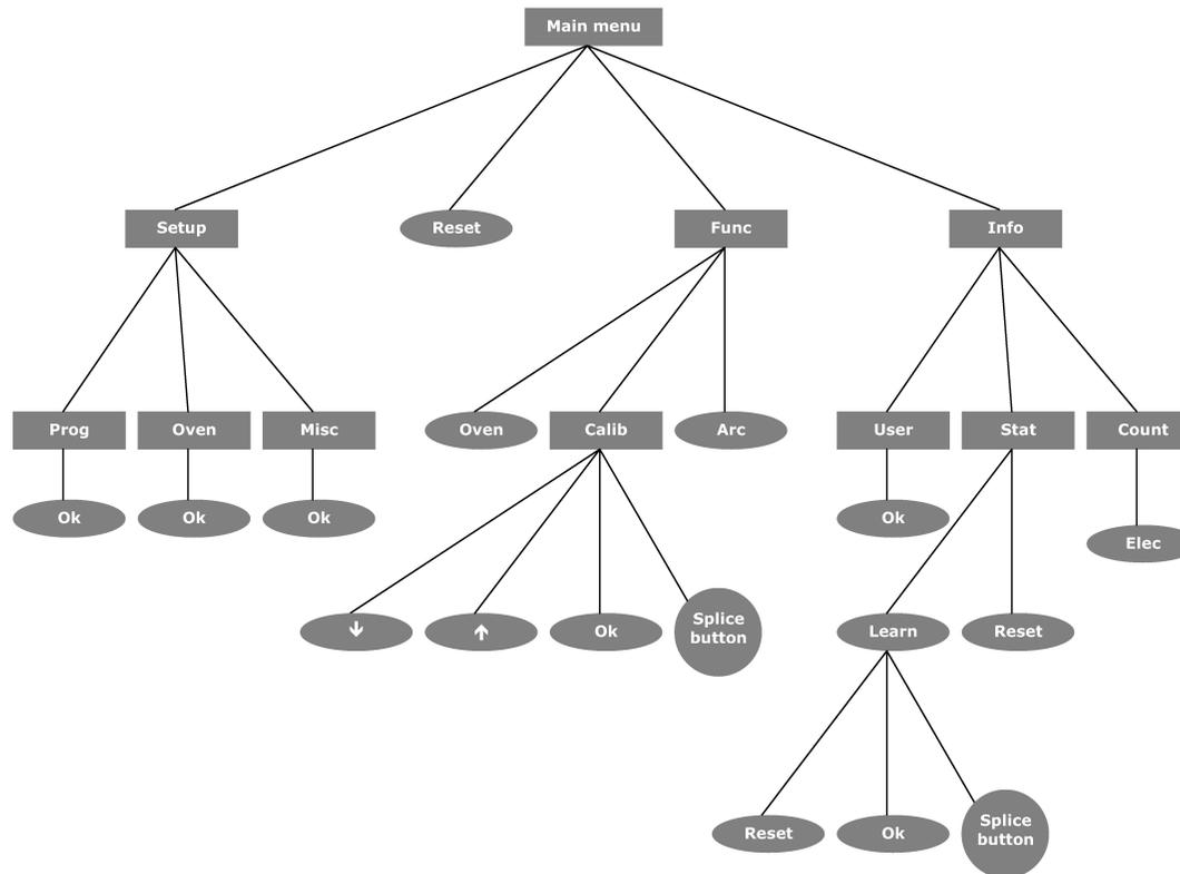
**Figure 3. Accessible commands from the fusion splicer menus**
