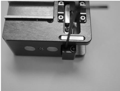
**Figure 34. Cleaving blade adjustment**
