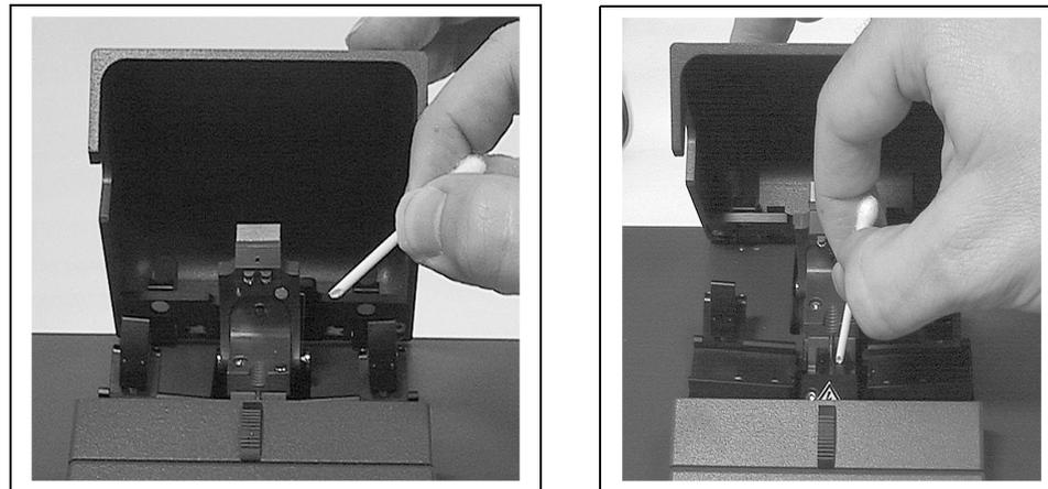
Figure 35. Cleaning the v-groove
