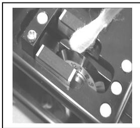
**Figure 28. Cleaning of the cleaver blade**
