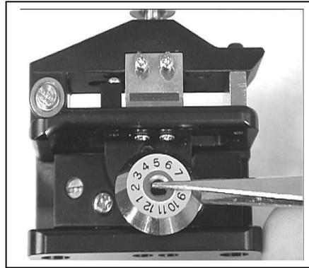
**Figure 32. Removal of the cleaver blade**
