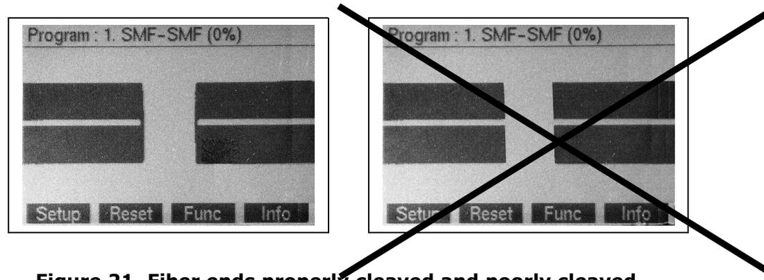
**Figure 21. Fiber ends properly cleaved and poorly cleaved**
