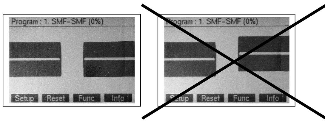
**Figure 22. Fibers properly aligned and fibers not properly aligned**
