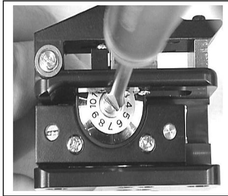
**Figure 31. Loosening of the cleaver blade**
