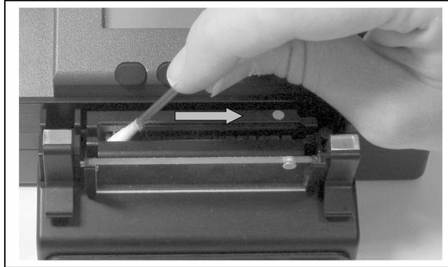
**Figure 36. Lubricating the oven with silicon grease**
