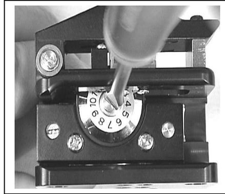
Figure 29. Loosening of the cleaver blade
