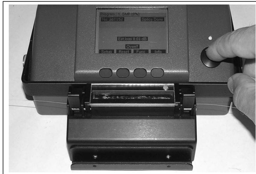
**Figure 27. Oven ready for operation. Press the splice/oven button to start the heat oven**
