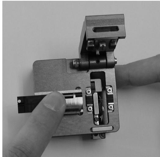
Figure 16. Loading the cleaver
