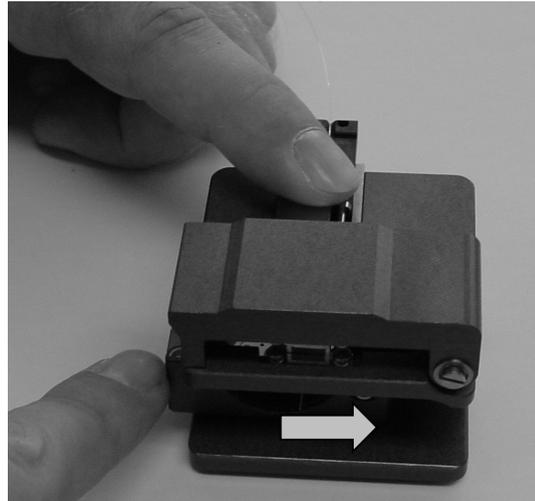
**Figure 17. Scoring and cleaving the fiber.**
