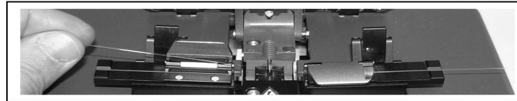
**Figure 25. Remove the fiber with open fiber holders**
