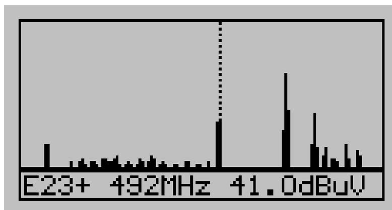
The meter shows the frequency spectrum of 48-860 MHz. A marker can select a certain channel (with the “UP”, “DOWN” buttons). Signallevel (in dBuV) of that channel will be shown in the display also.
