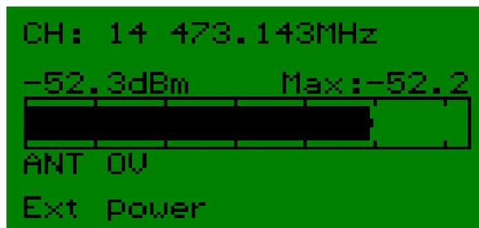
It is very easy to point an antenna towards a transmitter in this mode. The “maxhold function” (small bar in the big bar) will make it very accurate.
