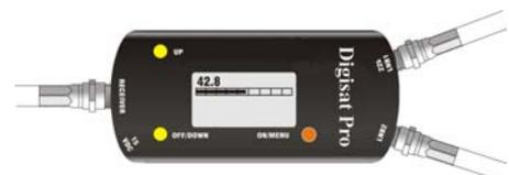
Note that you must select only one LNB to receive video signals for a viewable picture. The DIGISAT PRO ACCU is effectively dividing its attention to both ports LNB1 and LNB2 when both graphs are presented. This is perfect for dish alignment but interrupts the data stream to the receiver and it will present no video in this mode.
