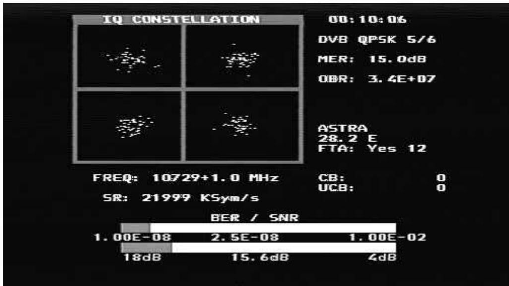
**Search +/-)** A signal search can be initiated by using the keypad '1 Search +' to search with increasing frequency or '2 Search -' with decreasing frequency. The search mode moves to the next peak in the spectrum and attempts a lock for DVB-S QPSK, DVB-S2 QPSK and DVB-S2 8PSK signals. The symbol rate is determined automatically. Because the time to lock for low symbol rate signals increases the lower the symbol rate, symbol rate signals below about 16000 will not lock during a search.
